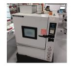
**Temperature Chamber** Thermotron temperature chamber for characterising devices over temperature. Capable of operating
