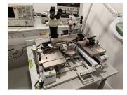
**RFOW** RF-on-wafer (RFOW) testing is carried out using a manual probe station. Up to two RF and two DC probes can be fitted.
