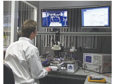
▲ Fig. 2 Evaluation of a mm-wave amplifier MMIC in Plextek's RFOW test laboratory.
