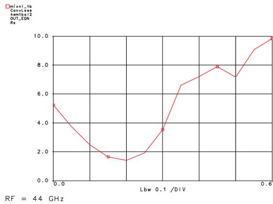
**Figure 4: Simulated Conversion Loss (dB) vs. Bondwire Inductance (nH) at 44 GHz**
