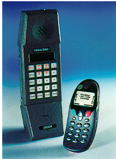
Figure 1: Size comparison of an early first generation cellular handset to today's (1997) leading edge second generation designs
