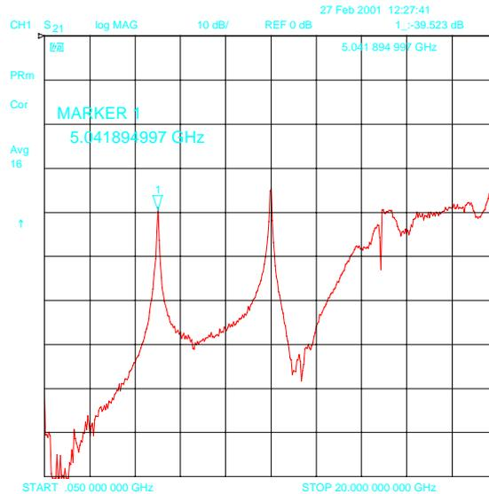
**Figure 9: Dupont 943, Ag metallisation, 5GHz resonator**
