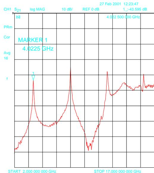
**Figure 8: Dupont 943, Ag metallisation, 4GHz resonator**
