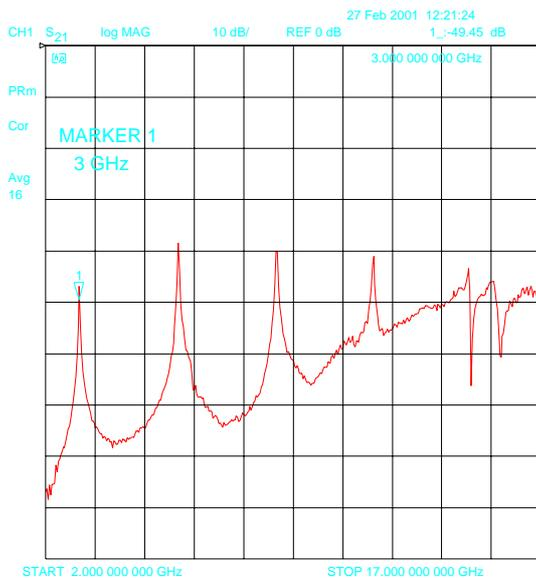
**Figure 7: Dupont 943, Ag metallisation, 3GHz resonator**
