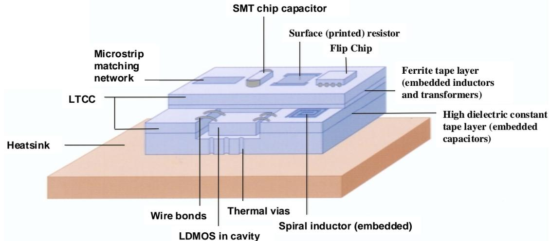
**Figure 1: LTCC substrate with integrated passives**
