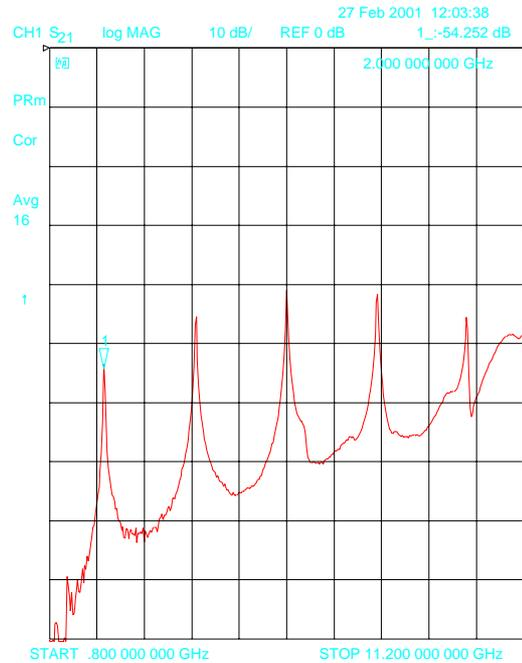
**Figure 6: Dupont 943, Ag metallisation, 2GHz resonator**
