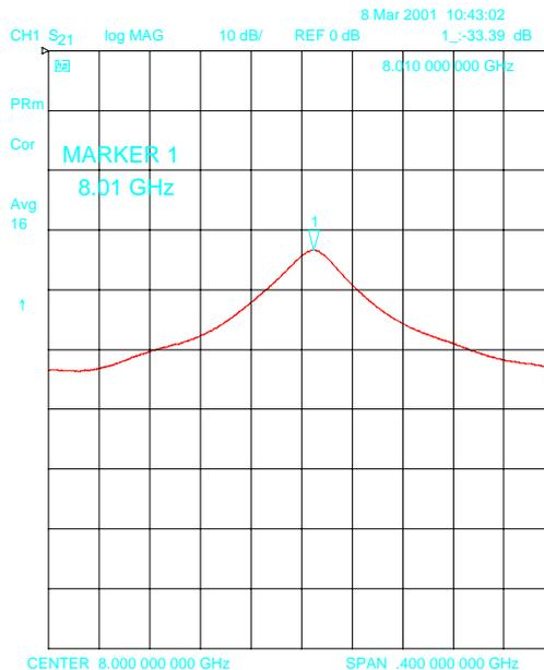
**Figure 10: Close-in plot of the 2<sup>nd</sup> harmonic of the 4GHz resonator on Dupont 943, Ag**
