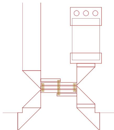
**Figure 26: Close-in of layout detail of the 22GHz to 35GHz Lange coupler**
