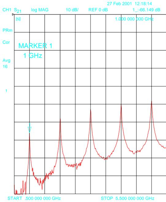
**Figure 5: Dupont 943, Ag metallisation, 1GHz resonator**
