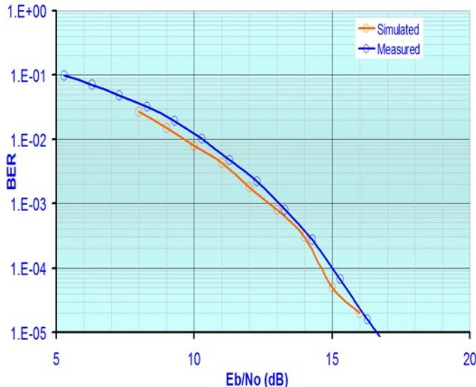
An excellent correlation was achieved between simulation and measurements as is clear from the graph above. Assuming a 6dB receiver noise figure, the sensitivity for 0.1% BER is 94.8dBm at nominal IF and deviation, improving to 96.7dBm at maximum deviation.
