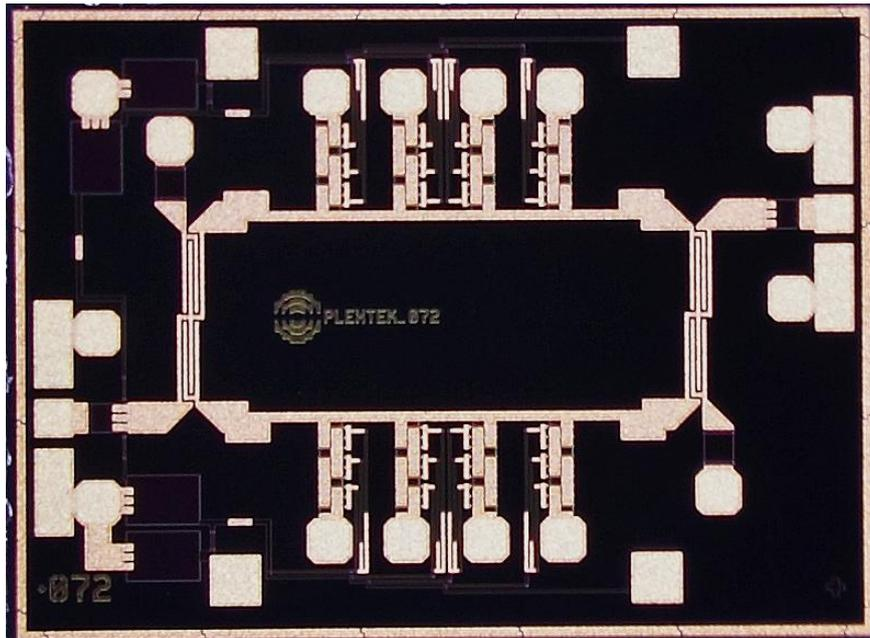
**Figure 9: Photograph of the balanced E-band VVA**
