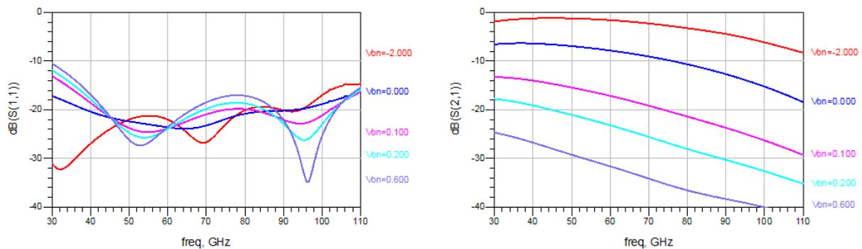
**Figure 6: Simulated small-signal performance of the balanced VVA**
