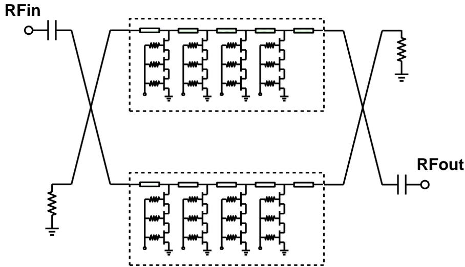
**Figure 5: Schematic of the balanced E-band VVA**
