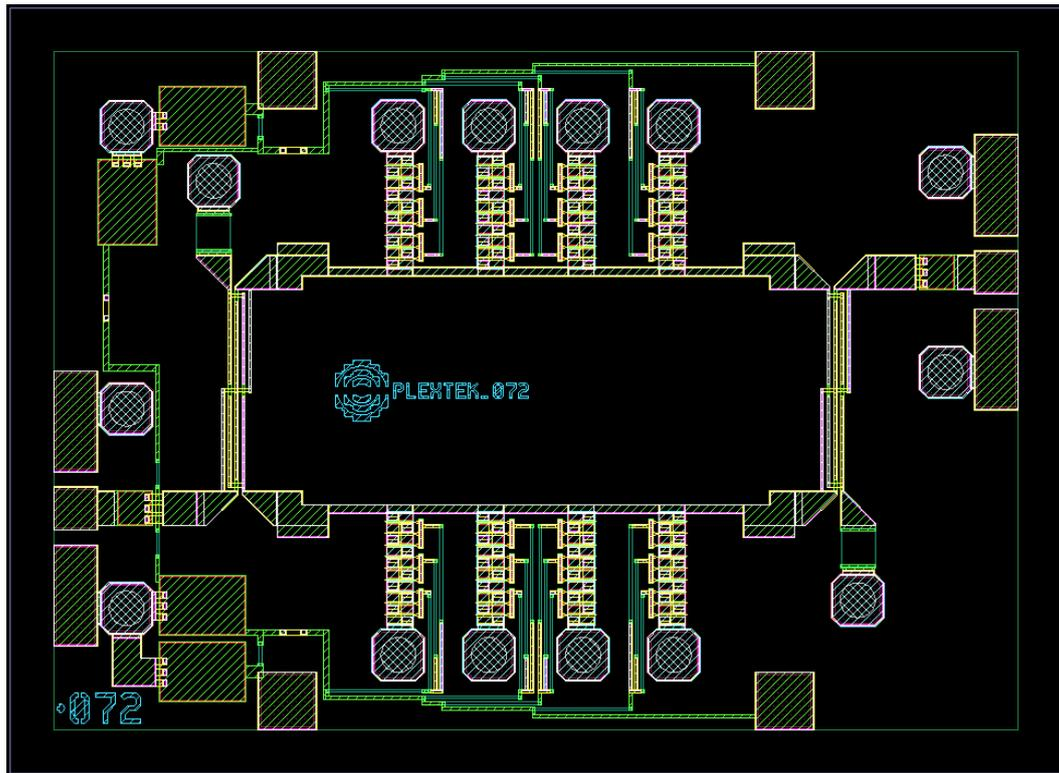
**Figure 8: Layout of the balanced E-band VVA**
