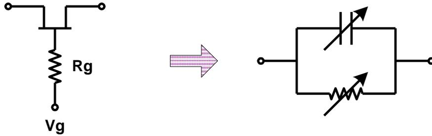
**Figure 2: Simplified equivalent circuit model for a zero-biased PHEMT**
