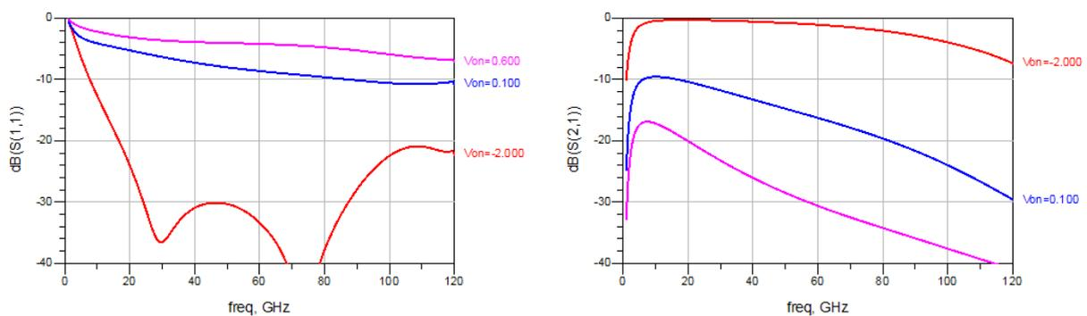
**Figure 4: Simulated small-signal performance of the core VVA**
