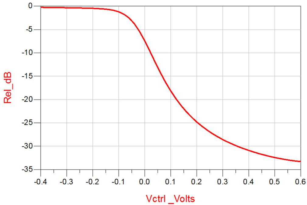
**Figure 7: Control voltage versus relative attenuation at 80GHz for the balanced VVA**
