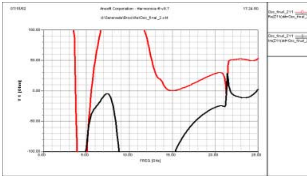
Figure 9: Simulated broadband response of 21.3GHz oscillator
