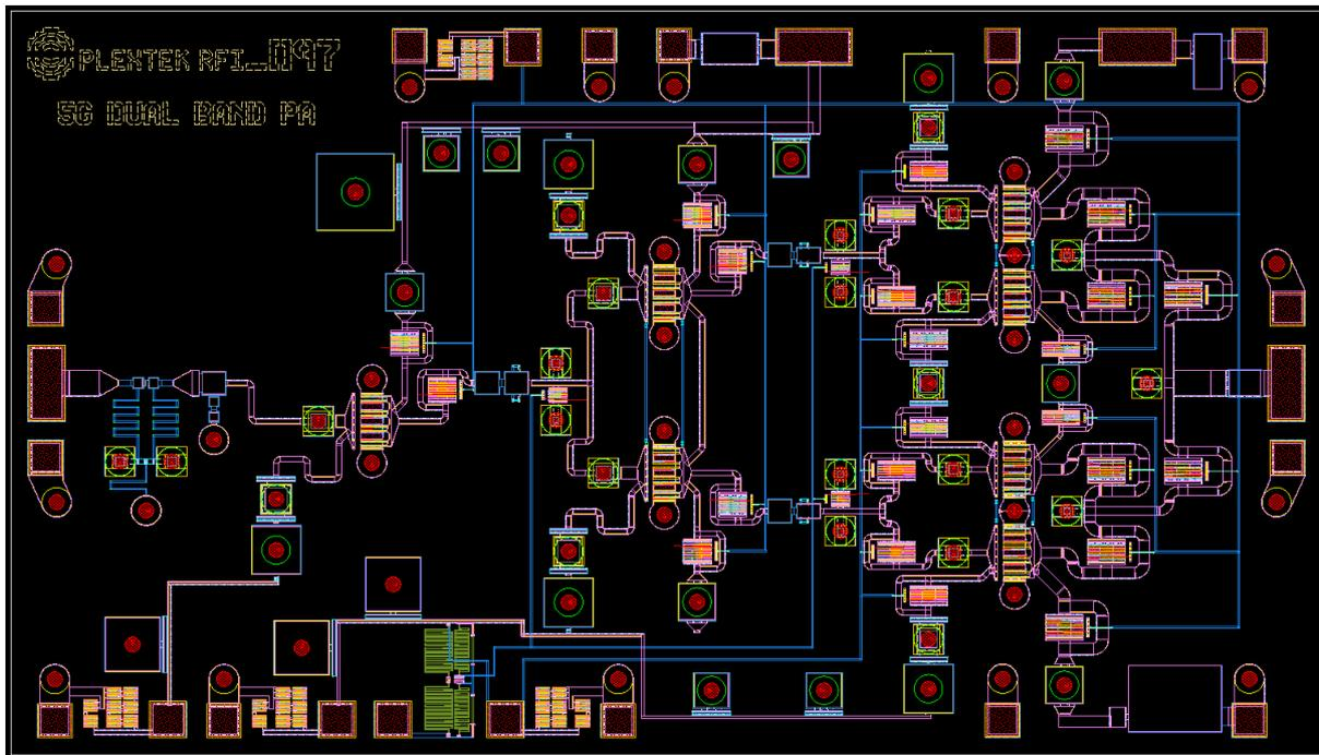
**Figure 1: Layout plot of one channel of the dual-band PA IC**
