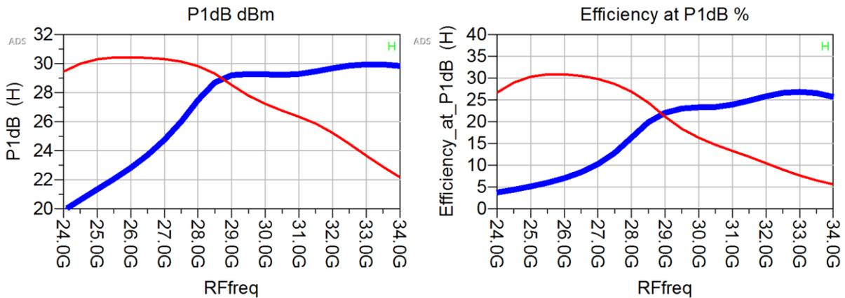
**Figure 6: Simulated large signal performance of the dual-band PA**
