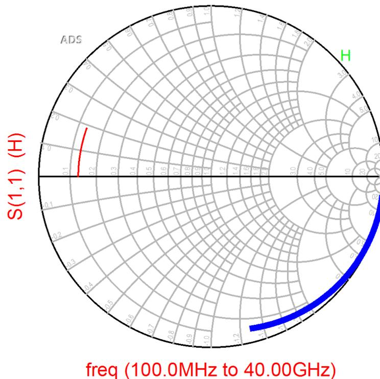
**Figure 4: Drain-source impedance of a  $4 \times 50 \mu\text{m}$  PHEMT in the on-state and off-state**
