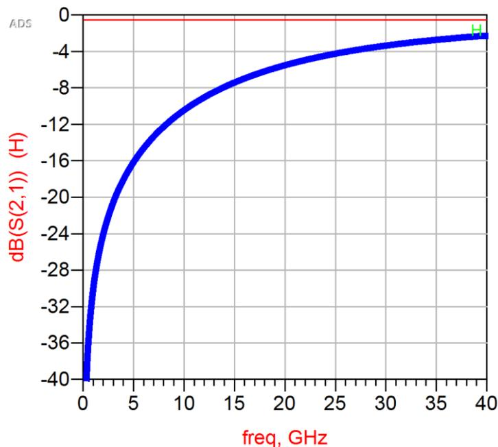
Figure 3: On-state and off-state insertion loss of a  $4 \times 50 \mu\text{m}$  PHEMT
