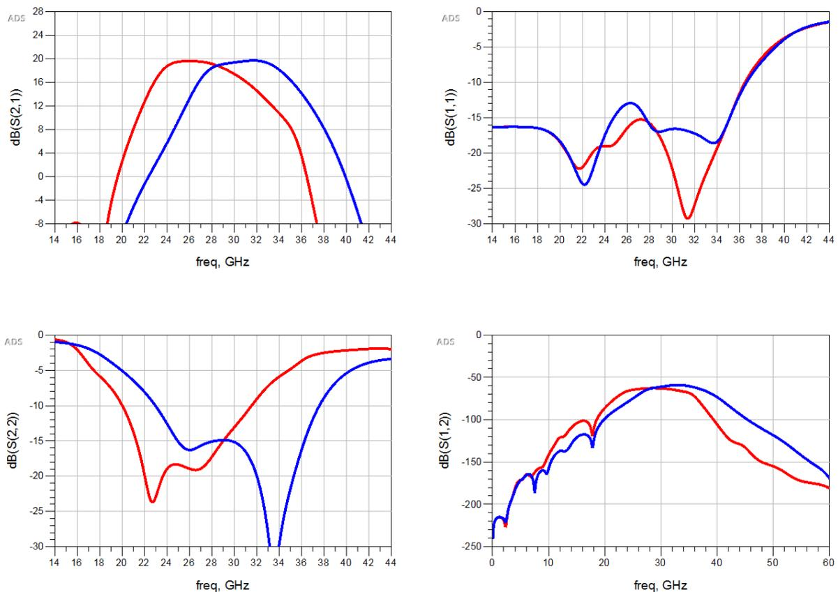
**Figure 5: Simulated s-parameters of the dual-band PA**
