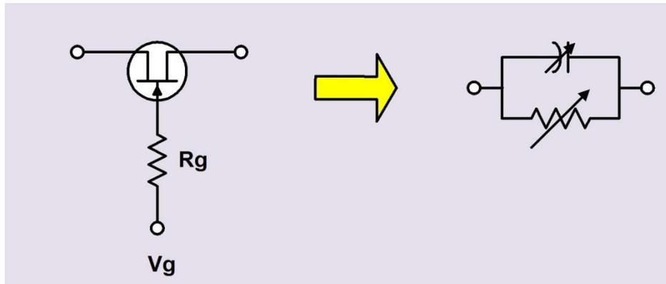
Figure 2: Simple equivalent circuit of a PHEMT as an RF switch
