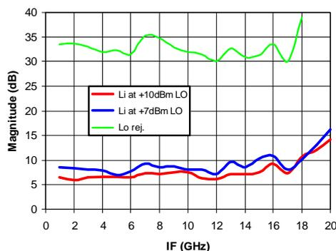
**Fig. 14. Measured conversion loss and LO rejection of the upconverter IC**
