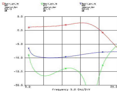
**Fig. 10. Two-port simulation of the active balun**
