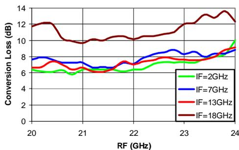
**Fig. 15. Measured conversion loss across RF band**
