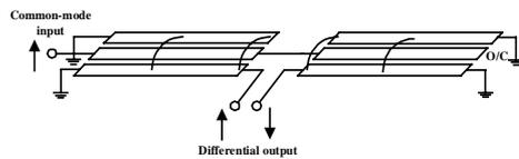
**Fig. 5. Multiple coupled line Marchand balun**
