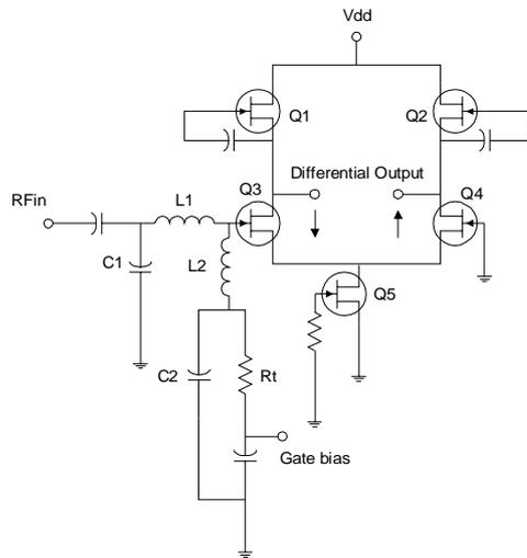
**Fig. 9. Input stage of IF active balun**
