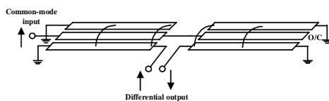
**Fig. 5. Multiple coupled line Marchand balun**
