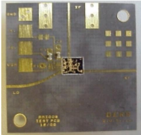
**Fig. 13. Photograph of an IC assembled onto a carrier**
