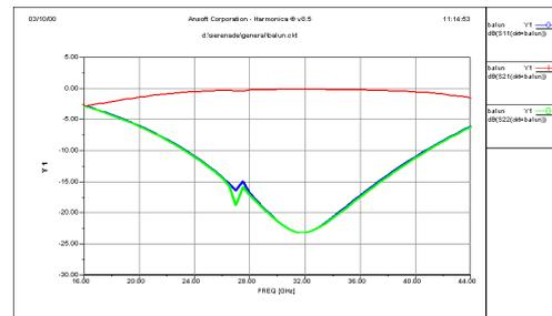
**Fig. 8. Electromagnetic 2-port simulation of the LO balun**
