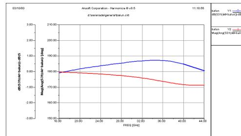
**Fig. 7. Electromagnetic simulation of amplitude and phase difference of the LO balun**
