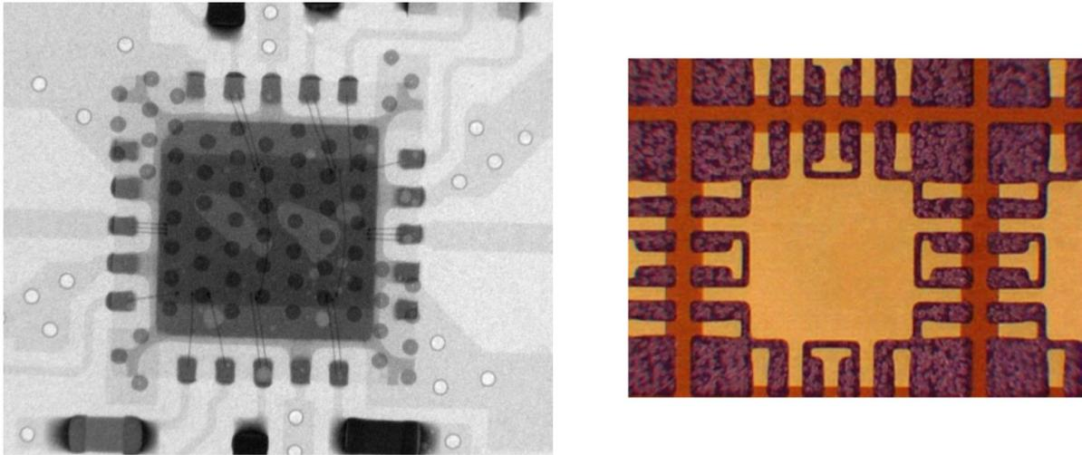
**Figure 10: Examples of custom leadframes for improved mmWave performance**
