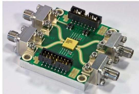
**Figure 13: Photograph of a laminate packaged dual channel 26GHz PA**
