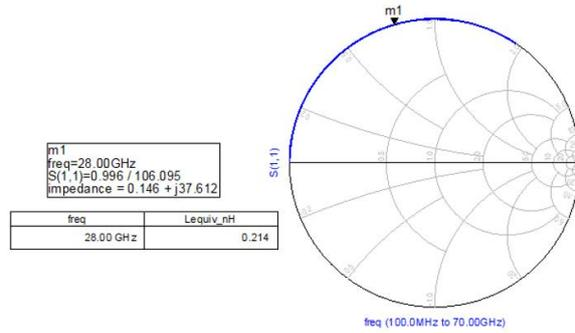
Figure 6: Simulated inductance of 3 short bonds
