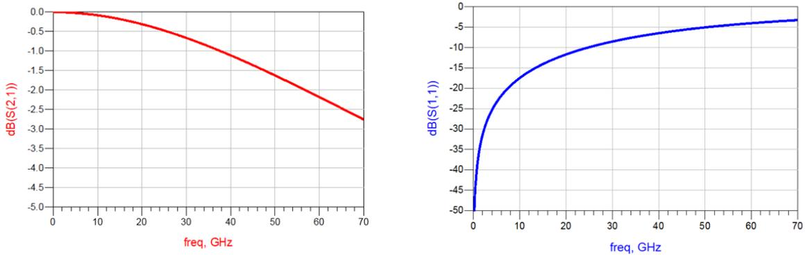
Figure 7: Simulated s-parameters of 3 short bonds as a series element
