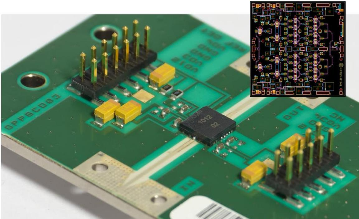
Figure 11: Photograph of a 39GHz PA in a 5mm x 5mm air cavity QFN with eval PCB
