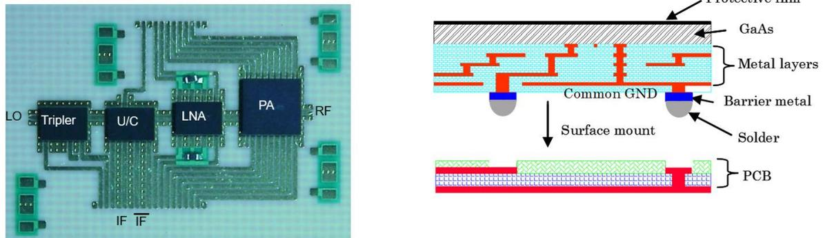
Figure 17: WLCSP evaluation PCB (LHS) and process cross-section (RHS) – courtesy Sumitomo
