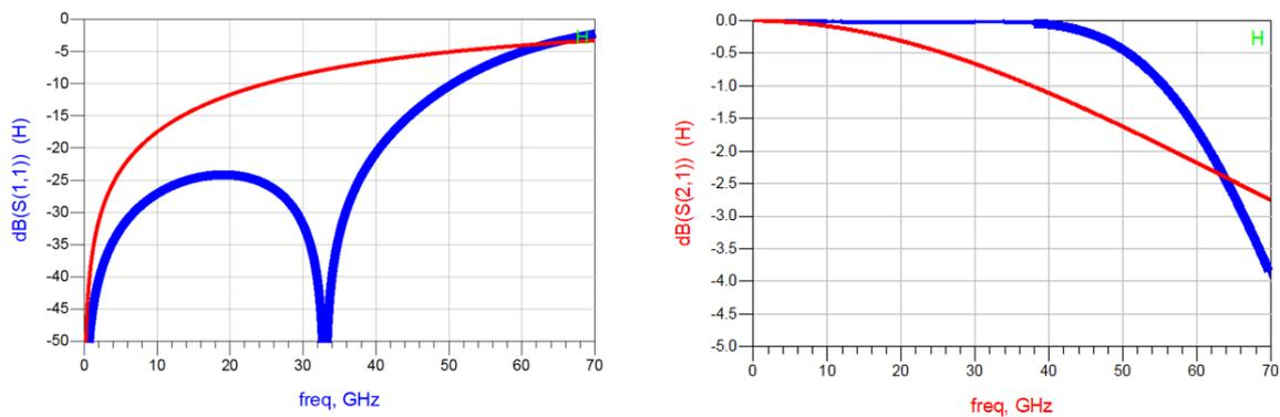
**Figure 8: Effect of adding capacitive compensation to the 3 bondwire connection**
