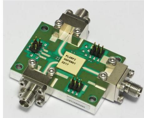
**Figure 12: Photograph of 26GHz FEM in 10mm x 10mm custom laminate SMT package**
