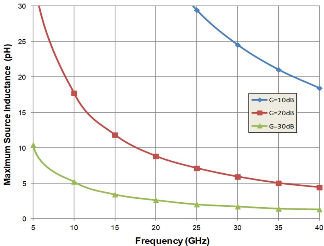
**Figure 4: Approximate levels of tolerable ground inductance versus frequency**
