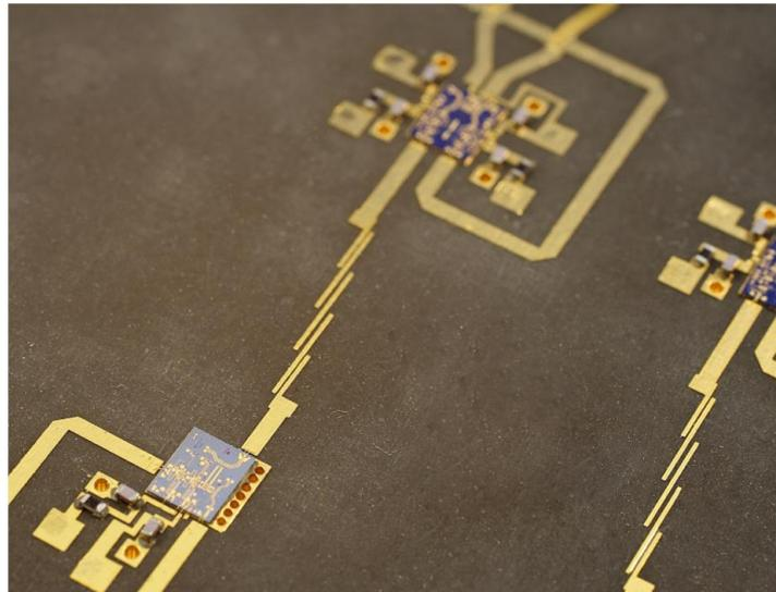
Figure 14: MMWave MCM with die mounted on the surface of a PCB
