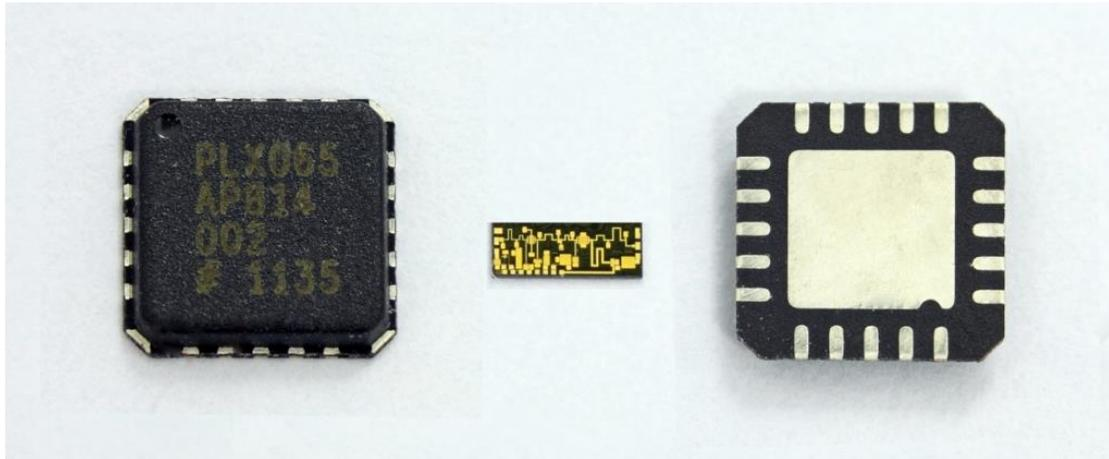
**Figure 2: Plastic over-moulded 5mm x 5mm QFN-20 package**
