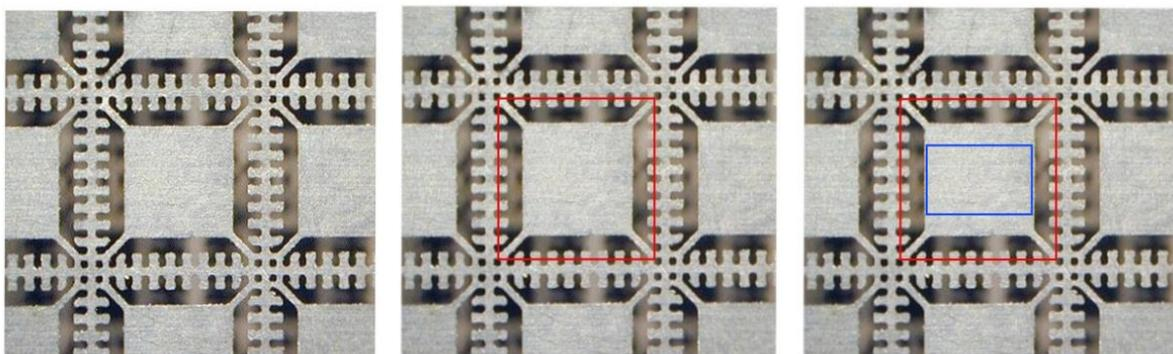
**Figure 3: Standard leadframe for 20 pin 5mm x 5mm QFN, with annotation**
