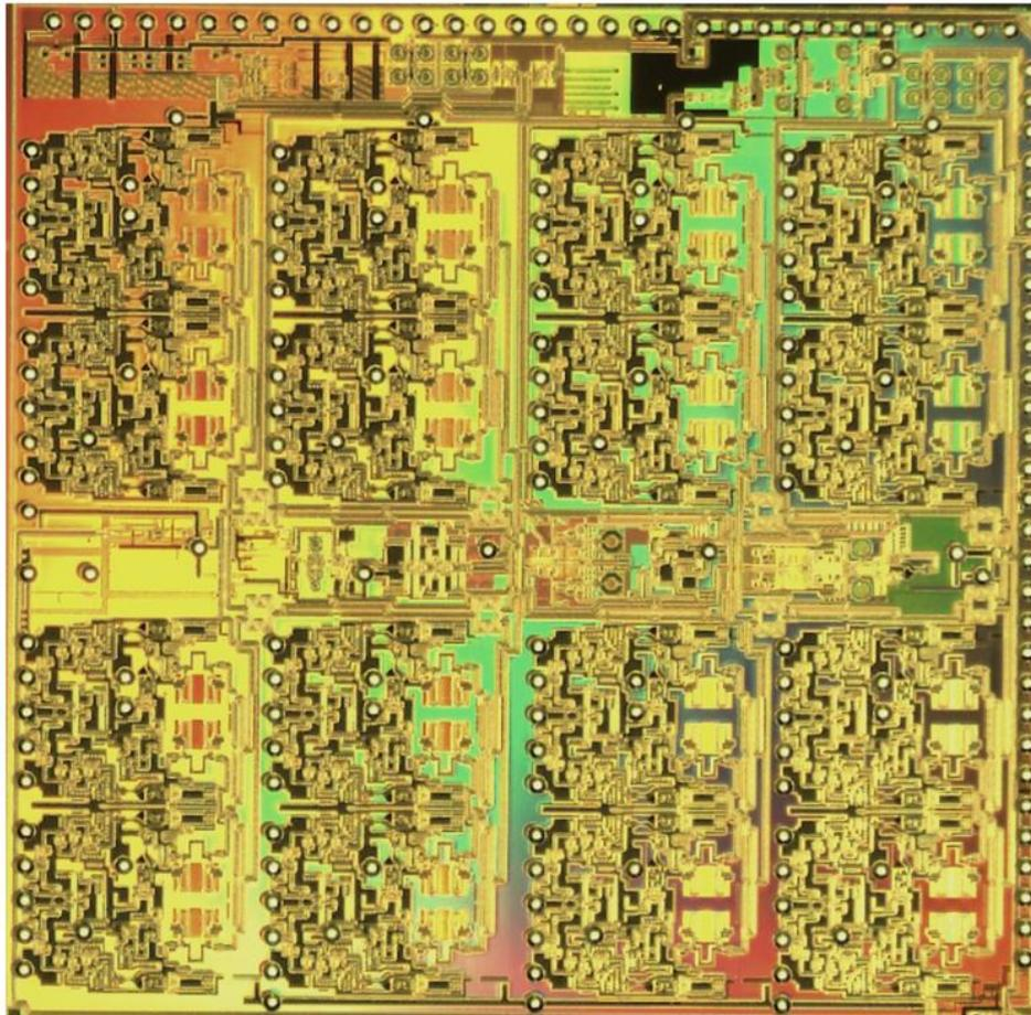
Figure 16: W-band phased array transceiver – courtesy of IBM
