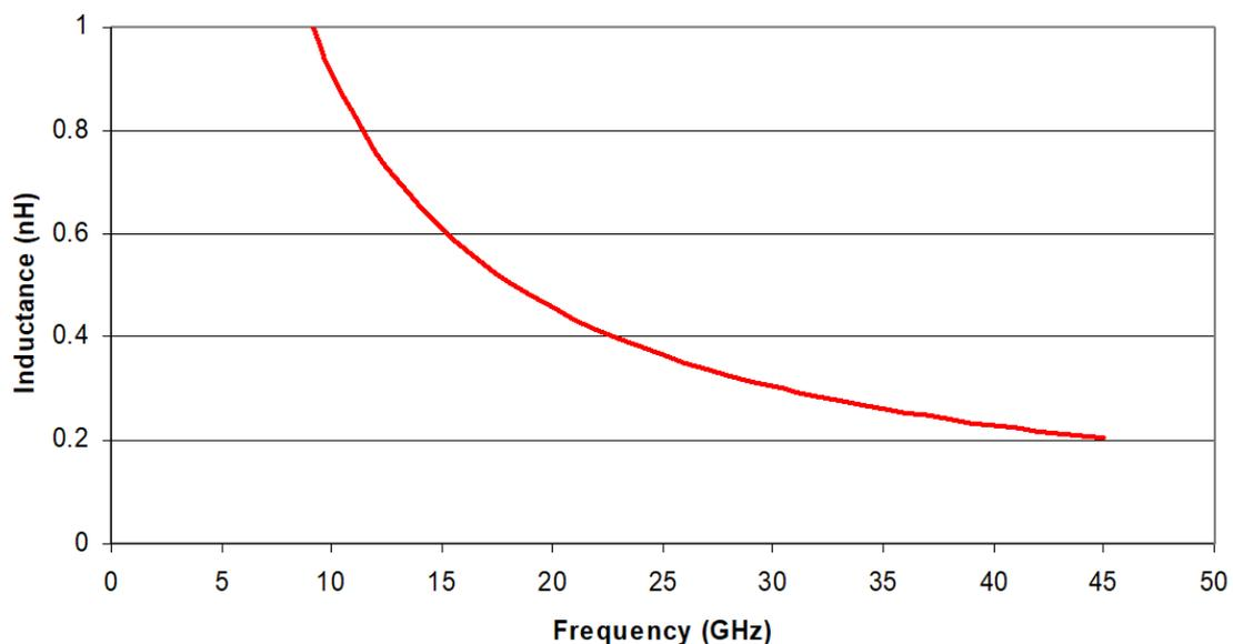
**Figure 9: Maximum inductance that can be perfectly compensated versus frequency**
