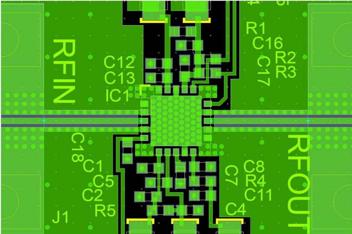
Figure 5: Example PCB layout with good RF grounding (courtesy of CML)
