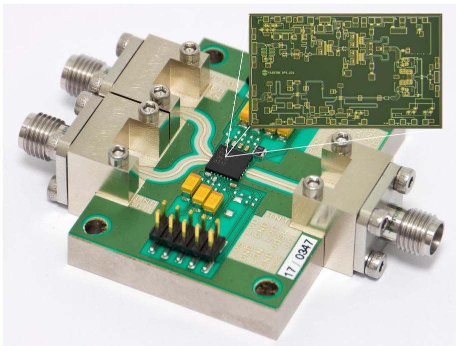
**Figure 1: 28GHz single chip FEM in over-moulded SMT package on eval PCB**
