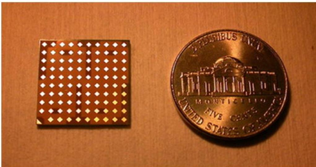
Figure 15: AiP package containing 4 transceiver die (64 radiating elements)
